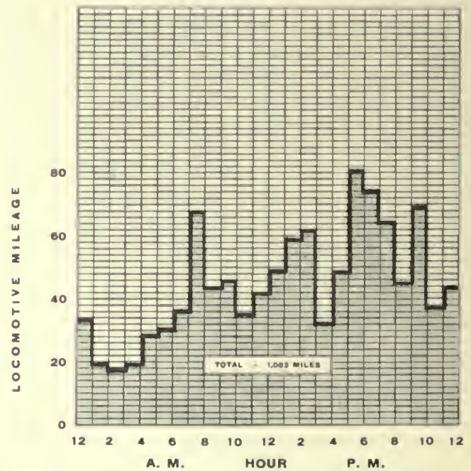
FIG. 406. TRAFFIC DIAGRAM. Locomotive-Mileage for the Average Day for Steam Operation in Passenger Transfer Service within Area of Investigation.
